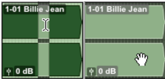
Smart Tool Select and Grab work on the tops and bottoms of clips.
